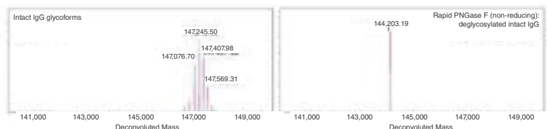
ESI-TOF analysis of an antibody before and after treatment with Rapid PNGase F (non-reducing format).
