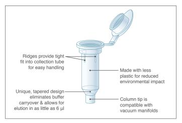
Our optimized column design supplied with the Monarch Gel Extraction and PCR & DNA Cleanup Kits enables elution in as little as 6  $\mu$ l, and eliminates buffer retention
