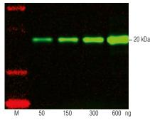
Typical SDS-PAGE of SNAP-Vista Green labeled proteins visualized using a gel scanner (Tyhoon 9400).
