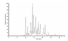
One hundred fmol of resuspended peptide mix may be analyzed by reverse phase liquid chromatography with on-line MS/MS analysis, for example with a Proxeon EASY-nLC and by Orbitrap Mass Spectrometer. Both analytical methods reveal a range of peptides in the standard. At least sixty percent sequence coverage is seen after database search, with greater than 15 unique peptides being identified.
