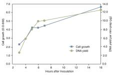
Miniprep DNA can be prepared from a single overnight colony after inoculation and only 3 hours growth. DNA yield doubles after an additional hour of growth.
