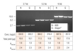
Monarch Plasmid Miniprep Kits consistently yield more concentrated plasmid DNA with equivalent purity and functionality as the leading supplier. Preps were performed according to recommended protocols using 1.5 ml aliquots of the same overnight culture. One microliter of each prep was digested with HindIII-HF (NEB #R3104) to linearize the vector and the digests were resolved on a 1% w/v agarose gel.
